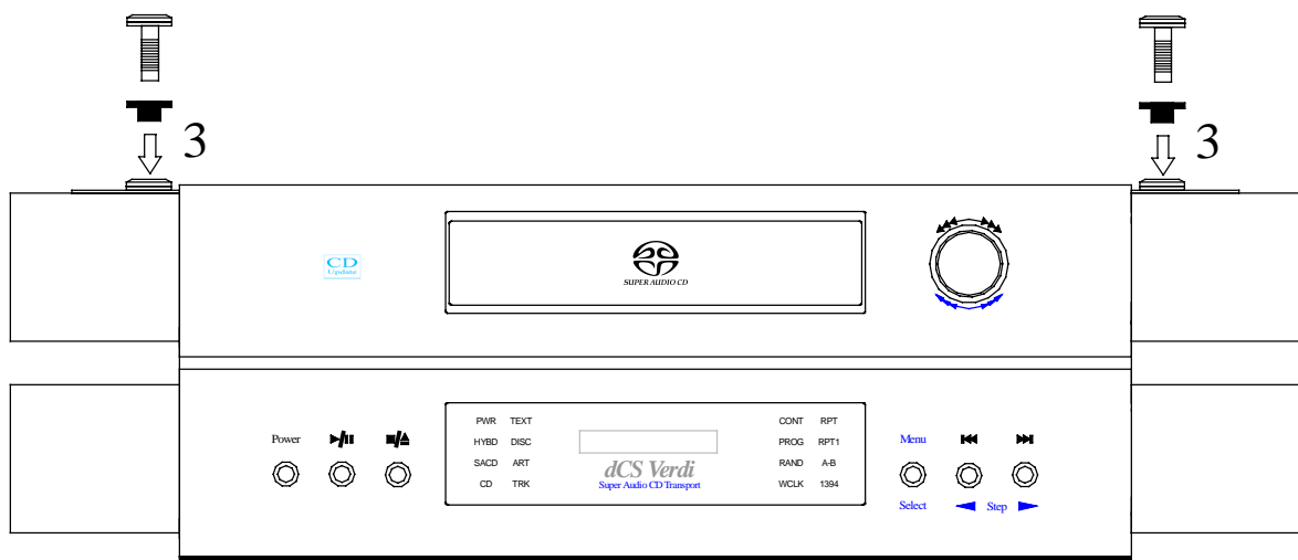
Figure 10 – Securing the Top Glass Plate
