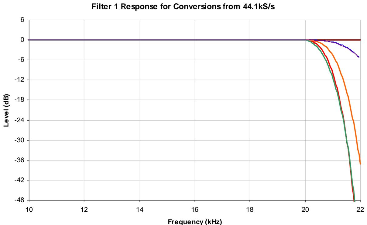
Figure 11 – Filter 1 Response Curves for Conversions from 44.1kS/s
