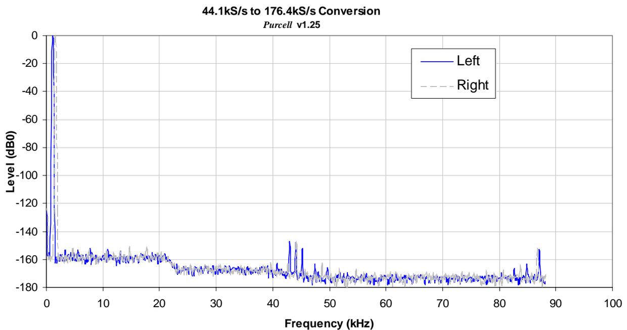
Figure 12 – Typical Spectrum for 44.1kS/s to 176.4kS/s Conversion
