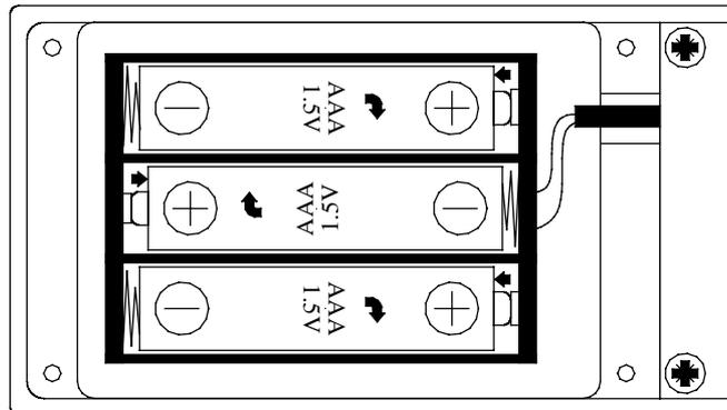
Figure 17 – Changing the Remote Control unit batteries
