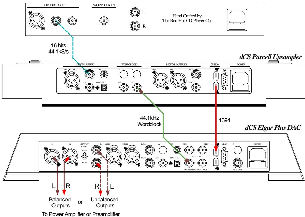
Figure 3 – Upsampling to DSD using an IEEE 1394 interface
