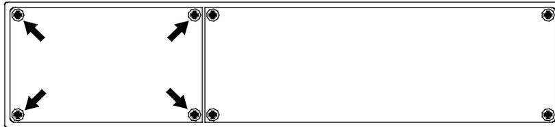
Figure 16 – Removing the Remote Control battery cover
